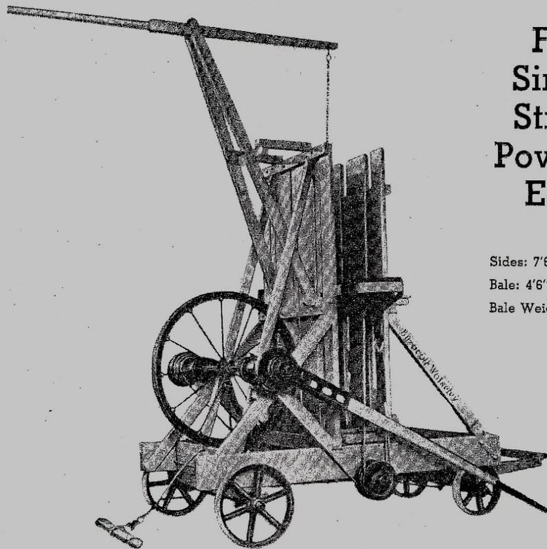
This press is horse-operated by means of whip attachment giving tremendous leverage, and doing away with hard manual work. After press is filled, the horse is hooked on and completes the pressing by walking away to the length of wire rope provided.
